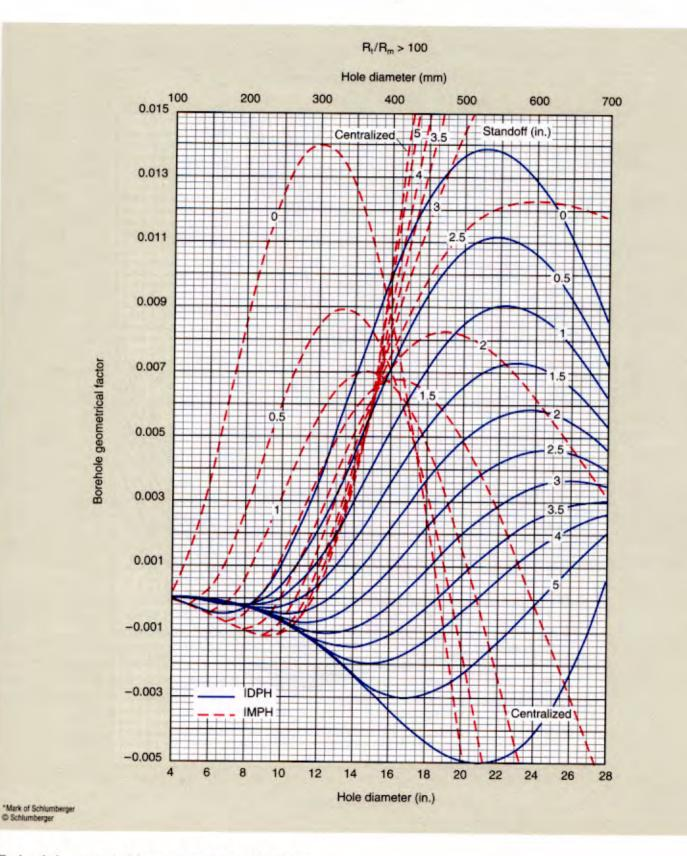
The borehole geometrical factor obtained from this chart or Chart Rcor-4c can be inserted into Nomograph Rcor-4a with the mud resistivity (R<sub>m</sub>) to determine the hole signal (in mS/m).
