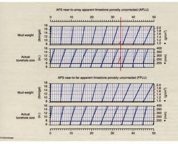
Charts Por-23a and -23b are used to apply environmental corrections to APLU and FPLU measurements.
