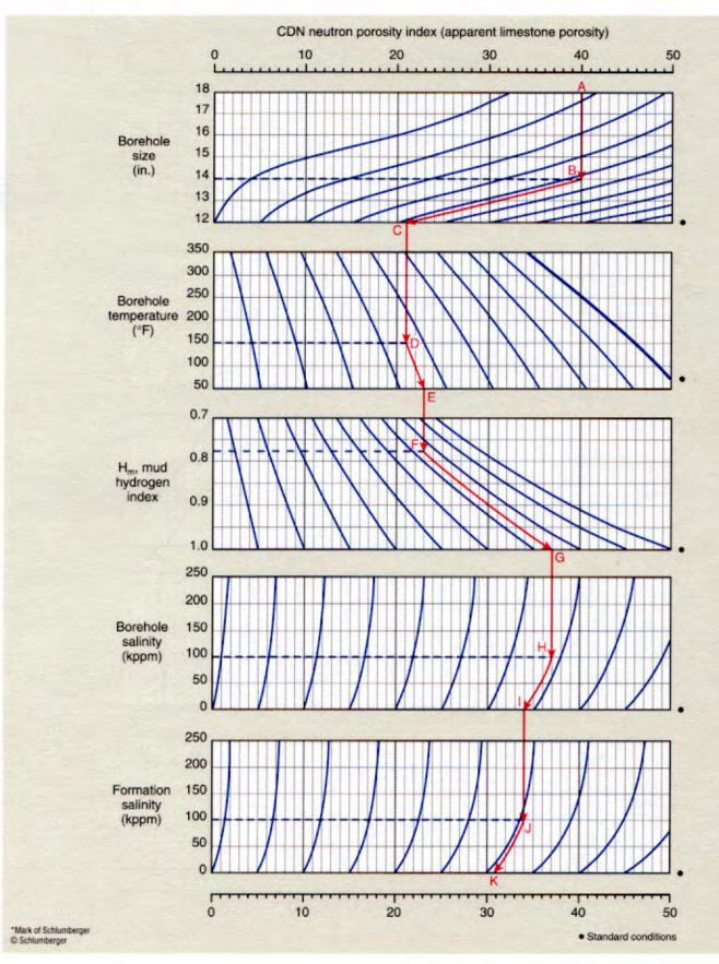
CDN\* Compensated Density Neutron Log Correction Nomograph for 8-in. Tool
