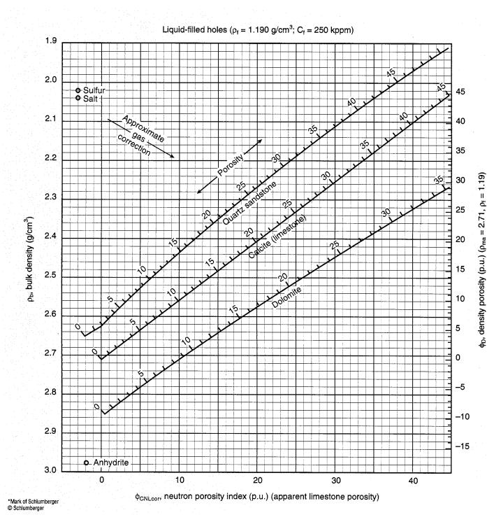
Porosity and Lithology Determination from Formation Density Log and CDN\* Compensated Density Neutron Log for 6.5-in. Tool
