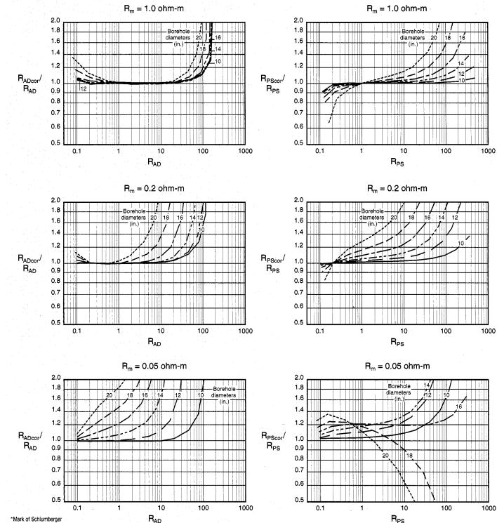
$R_{PS}$  is the apparent resistivity from the phase shift-shallow, and  $R_{AD}$  is the apparent resistivity from the attenuation-deep. Charts Rcor-11a, -11b and -11c provide borehole corrections for the 6.5-, 8- and 9.5-in. CDR tools run in mud resistivities
