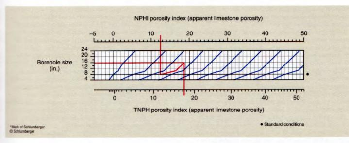
Enter the chart from the top at 12.5 p.u.; drop down to 7%-in. hole size, labeled with a bullet (•) for standard conditions. Follow the trend lines upward to 16 in. From that point drop straight down to the TNPH scale and read the uncorrected TNPH = 17.25 p.u. If NPHI is recorded in units other than limestone units, it must be converted using Chart Por-13 before it can be used in this chart. The NPHI scale is for use with logs recorded after January 1976.
