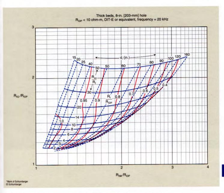
This chart uses the raw, unboosted induction signals and the ID Phasor value to define the invasion profile in a rock drilled with oil-base mud. To use the chart, the ratio of the raw, unboosted medium induction signal (IIM) and the deep Phasor induction (IDP) is entered in abscissa. The ratio of the raw, unboosted deep induction signal (IID) and the deep Phasor induction (IDP) is entered in ordinate. Their intersection defines  $d_i$ ,  $R_{xo}/R_t$  and  $R_t/R_{IDP}$ .
