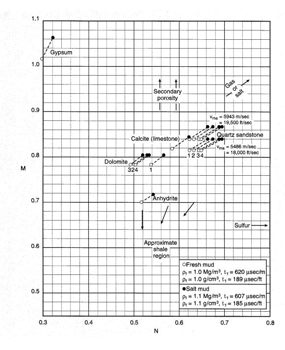
This crossplot may be used to help identify mineral mixtures from sonic, density and neutron logs. (The CNL neutron log is used in the above chart; the time average sonic response is assumed.) Except in gas-bearing formations, M and N are practically independent of porosity. They are defined as:
