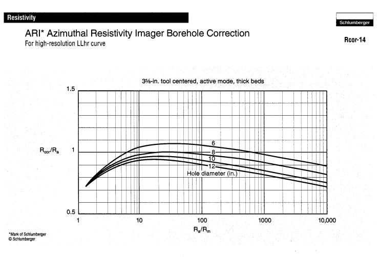
The high-resolution deep resistivity curve available from the ARI Azimuthal Resistivity Imager log is subject to borehole effects like any other laterolog measurement. Borehole correction is performed using Chart Rcor-14 in the same way as the deep and shallow laterolog borehole corrections and the microlog and MicroSFL\* mudcake corrections (see Charts Rxo-2 and Rxo-3 for an explanation and illustration).
