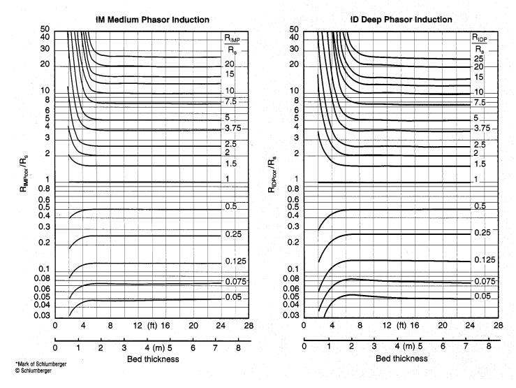
These charts (Rcor-9) correct the DIT-E Phasor Induction (IM and ID) measurements for bed thickness.
