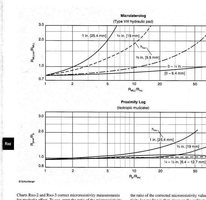
Charts Rxo-2 and Rxo-3 correct microresistivity measurements for mudcake effect. To use, enter the ratio of the microresistivity log reading divided by the mudcake resistivity into the abscissa of the appropriate chart. Go vertically to the mudcake thickness; the ratio of the corrected microresistivity value to the microresistivity log reading is then given on the ordinate. Multiplication of this ratio by the microresistivity log reading yields the corrected microresistivity.
