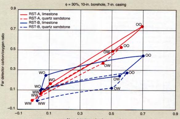
Near detector carbon/oxygen ratio
