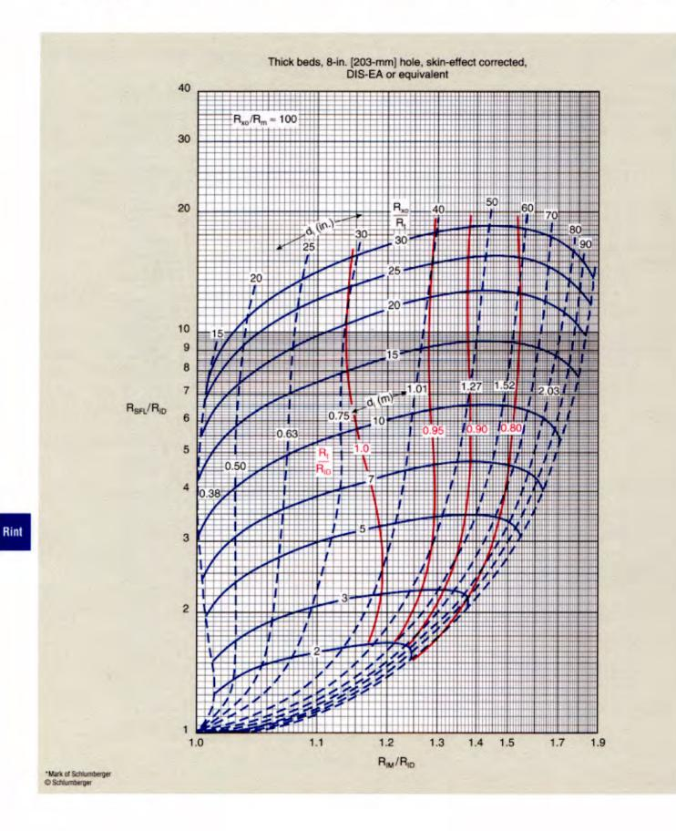
Deep Induction-SFL\* Spherically Focused Resistivity Log-R<sub>xo</sub> Device
