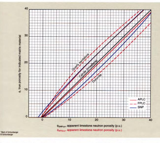
When the APS or SNP log is recorded in limestone porosity units, this chart is used to find porosity in sandstones or dolomites. First, correct the SNP log for mudcake thickness (Chart Por-15a).
