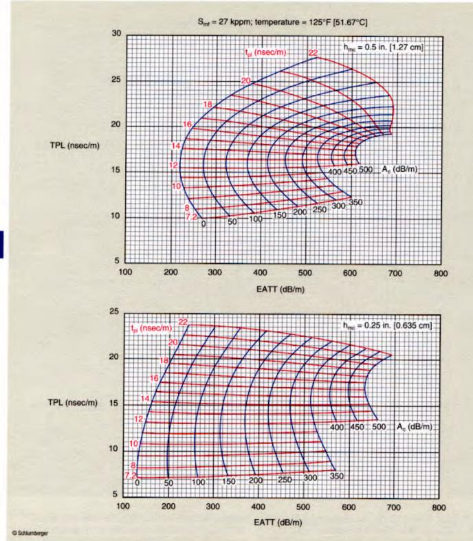
In general, low-conductivity muds produce the largest effects so that increases in temperature, mudcake porosity and salinity generally reduce the mudcake effects. The charts displayed here assume a mudcake porosity of 40 p.u. (For more information see Reference 31.) The mudcake thicknesses are estimated from a caliper or a Microlog using Chart Rxo-1.
