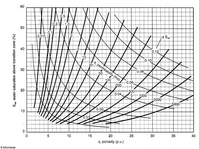
Charts K-3 and K-4 provide an estimate of permeability for sands, shaly sands or other hydrocarbon-saturated intergranular rocks at irreducible water saturation,  $S_{wi}$ . Both charts are based on empirical observations and are similar in form to a general expression proposed by Wyllie and Rose (1950):  $k^{1/2} = (c\phi/S_{wi}) + C'$ .
