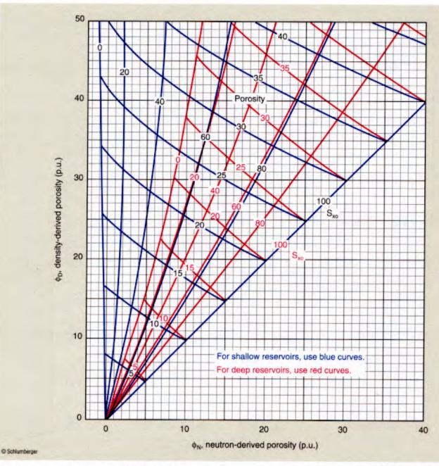
Based on reservoir depth and conditions, enter the appropriate chart with matrix-corrected porosity values. Average water saturation in the flushed zone,  $S_{xo}$ , and porosity are derived. This chart assumes fresh water and gas of composition  $C_{1.1}H_{4.2}$ , and it includes correction of the neutron log for "excavation effect."
