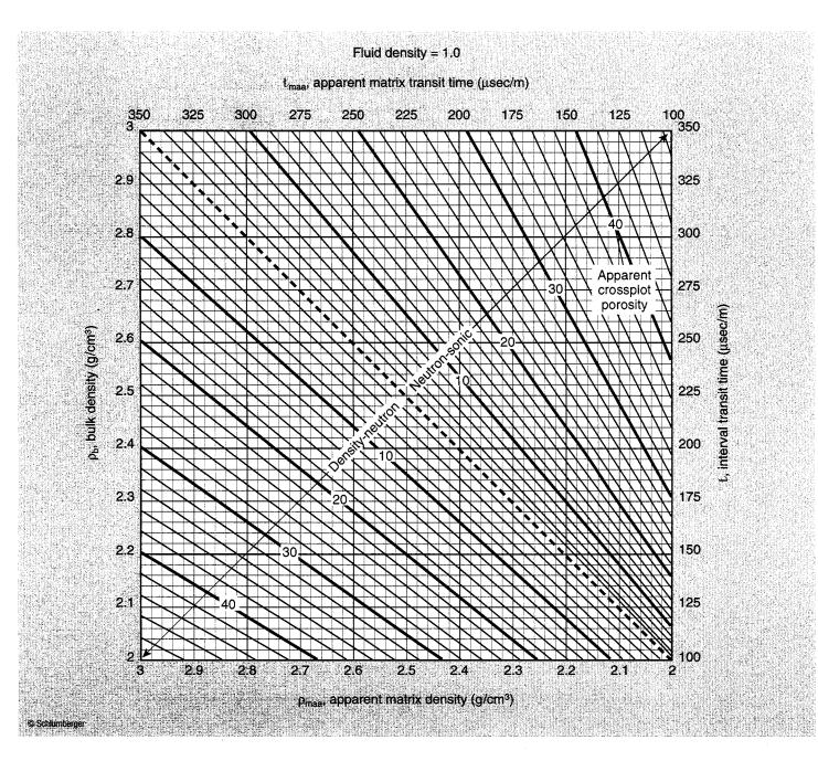
Next, enter the appropriate CP-14 chart with the interval transit time. Go to the apparent crossplot porosity previously found on the appropriate neutron-sonic crossplot chart. This defines an apparent matrix interval transit time,  $t_{maa}$ . Similarly, enter the same chart with the bulk density,  $\rho_b$ . Go to the apparent crossplot porosity previously found on the appropriate density-neutron crossplot chart. This defines an apparent matrix grain density,  $\rho_{maa}$ .
