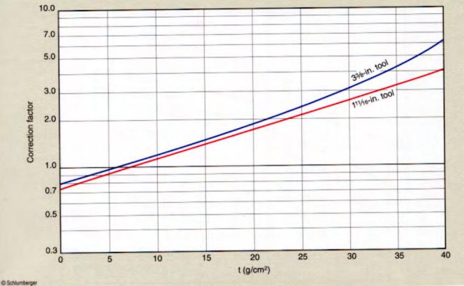
Log interpretation Chart GR-3 is based on laboratory work and Monte Carlo calculations to provide gamma ray corrections in cased holes. This chart is based on the openhole model in Chart GR-1. In this case, t, in g/cm2, is calculated as the sum of density-thickness products for the casing, cement sheath and borehole fluid. The density of J-55 casing is 7.96 g/cm3, and the density of cement is typically 2.0 g/cm3.
