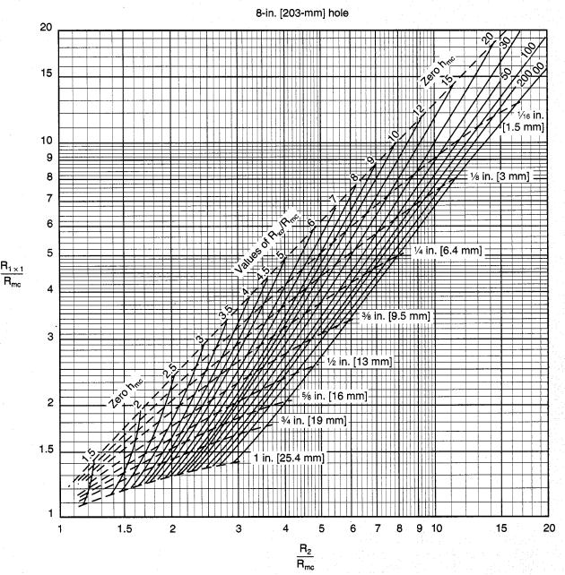
Enter the chart with the ratios  $R_{1\times 1}/R_{mc}$  and  $R_2/R_{mc}$ . The point of intersection defines the  $R_{xo}/R_{mc}$  ratio and the mudcake thickness,  $h_{mc}$ . Knowing  $R_{mc}$ ,  $R_{xo}$  can be calculated.
