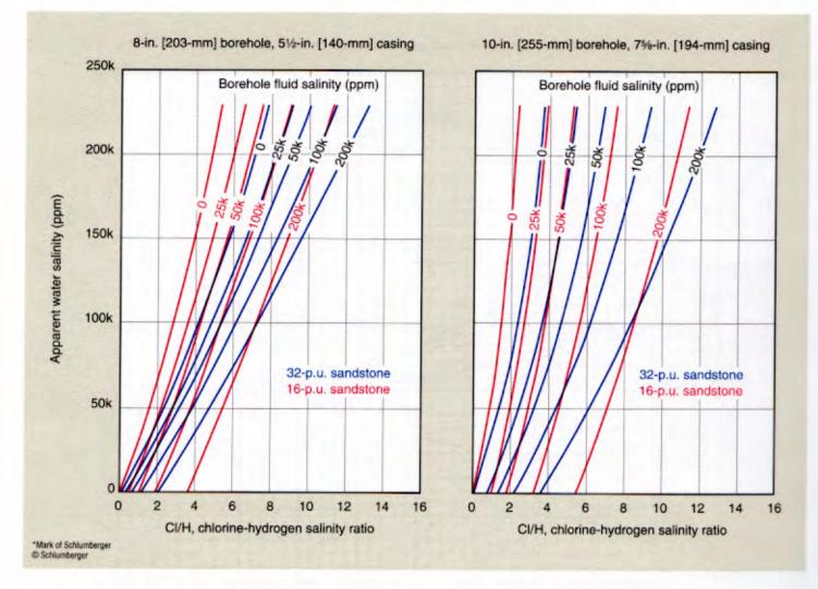
Charts GST-3 and GST-4 permit the determination of an apparent water salinity from the chlorine-hydrogen ratio (Cl/H) as recorded with the GST Induced Gamma Ray Spectrometry Tool. Two sets of charts are presented. Chart GST-3 applies when the GST tool is operated in inelastic mode; Chart GST-4 applies when the tool is operated in capture-tau mode.
