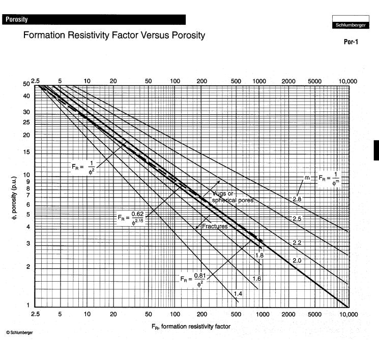
This chart gives a variety of formation resistivity factor-toporosity conversions. The proper choice is best determined by laboratory measurement or experience in the area. In the absence of this knowledge, recommended relationships are the following: For soft formations (Humble formula):
