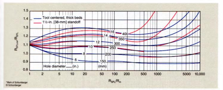
Most resistivity measurements should be corrected for borehole effect. Charts Rcor-1 and Rcor-8 provide the borehole correction for the 16-in. Normal and the SFL measurements.
