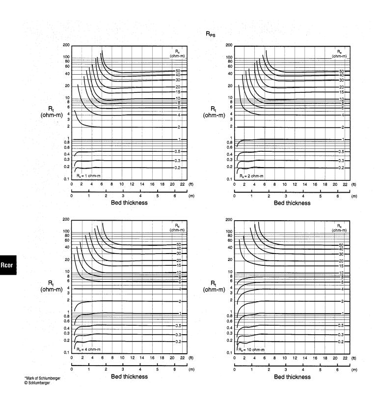
Charts Rcor-12 and Rcor-13 correct the CDR tool resistivities for bed thickness. To use, select the chart appropriate for the measurement ( $R_{PS}$  or  $R_{AD}$ ) and for the adjacent bed resistivity ( $R_{S}$ ). Enter the chart with the bed thickness, which can be determined from the distance between the crossovers of  $R_{PS}$  and  $R_{AD}$ . Proceed upward to the  $R_a$  curve corresponding to the center bed resistivity value. Read the corrected resistivity value  $(R_t)$  on the ordinate.
