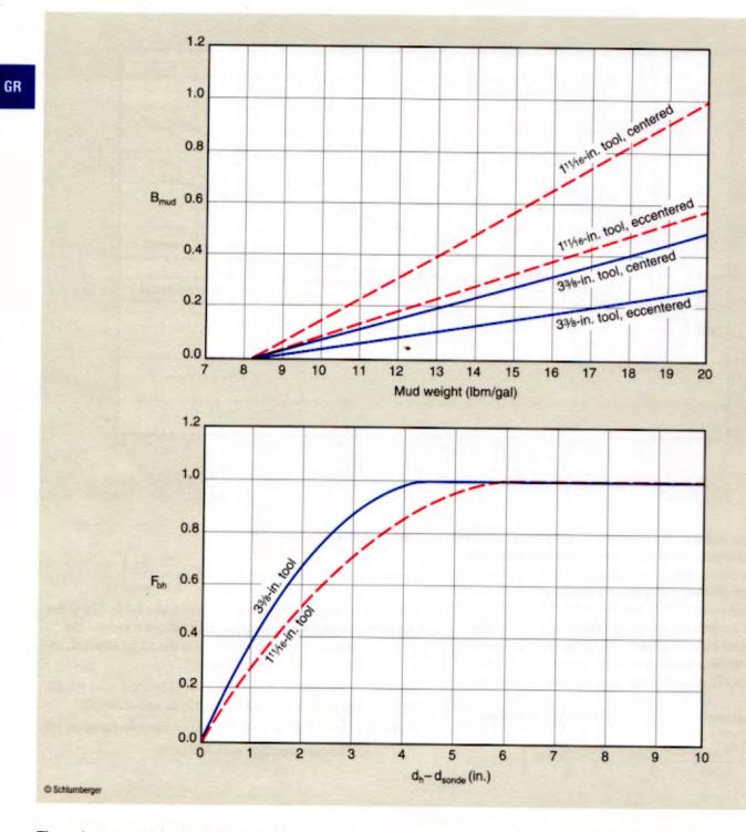
These charts correct for the barite mud effect in hole sizes smaller and larger than the 8-in. standard. In these cases, the correction factor from Chart GR-1 is multiplied by the borehole correction factor  $1 + B_{mud} \times F_{bh}$ .
