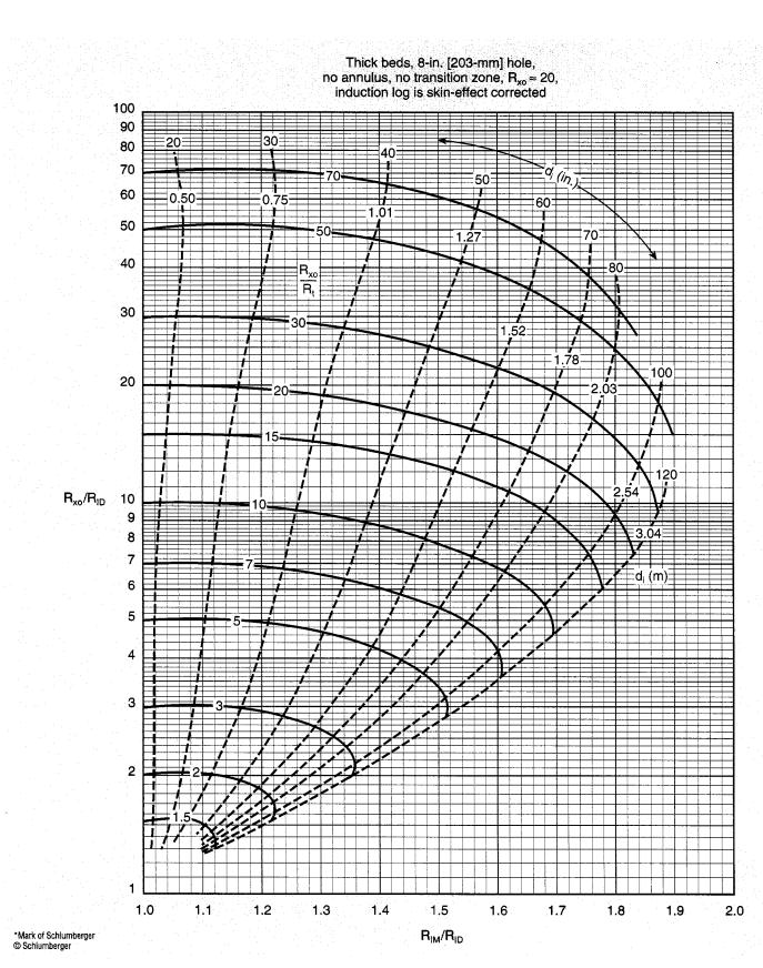
To use this chart in an oil-base mud environment, use synthetic R<sub>xo</sub> calculated from EPT\* or TDT\* logs.
