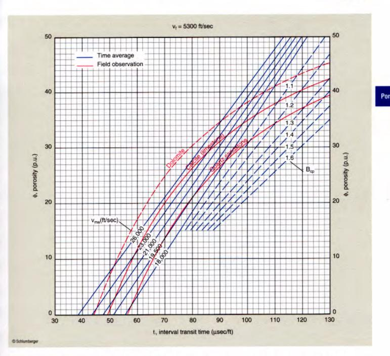
These two charts (Por-3) convert sonic log interval transit time, t, into porosity,  $\phi$ . Two sets of curves are shown. The blue set employs a weighted-average transform. The red set is based on empirical observation (see Reference 20). For both, the saturating fluid is assumed to be water with a velocity of 5300 ft/sec (1615 m/sec).
