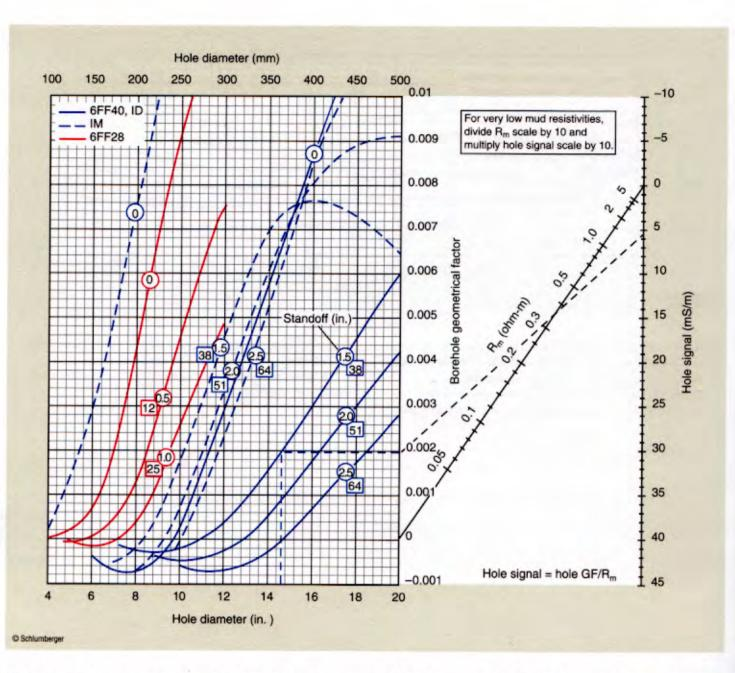
The hole-conductivity signal is to be subtracted, where necessary, from the induction log conductivity reading before other corrections are made.<sup>†</sup> This correction applies to all zones (including shoulder beds) having the same hole size and mud resistivity.
