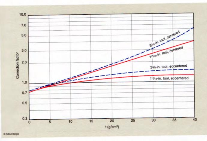
Log interpretation Charts GR-1 and GR-2, replacing Chart Por-7, are based on laboratory work and Monte Carlo calculations to provide improved corrections for 3<sup>3</sup>/<sub>4</sub>- and 1<sup>11</sup>/<sub>16</sub>-in. SGT gamma ray tools. The corrections normalize the response of both tools to eccentered positions in an 8-in. borehole with 10-lbm mud. Chart GR-2 provides a correction for barite mud in small boreholes.
