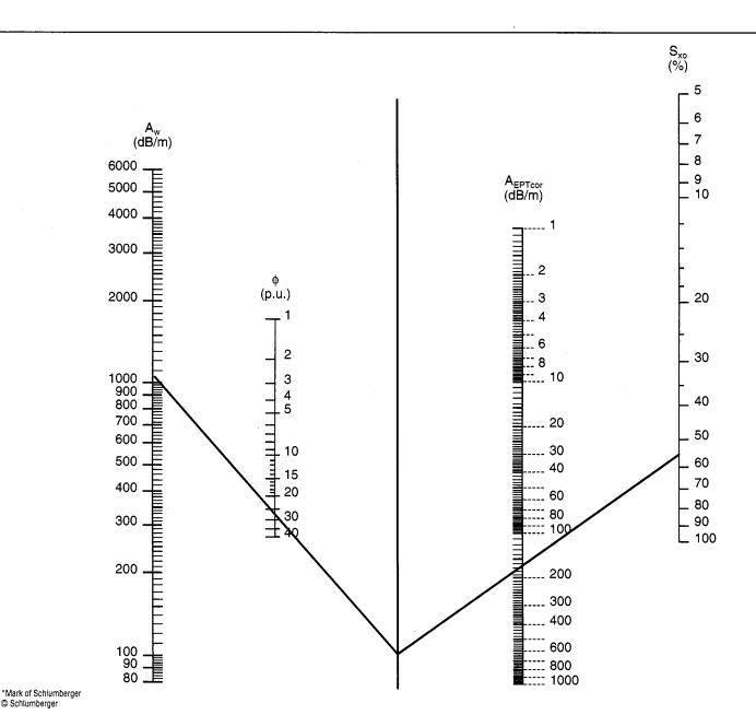
The nomograph defines water saturation in the rock immediately adjacent to the borehole,  $S_{xo}$ , using the EPT attenuation measurement. It requires knowledge of saturating fluid (usually mud filtrate) attenuation ( $A_w$ ), porosity and the EPT attenuation ( $A_{EPTcor}$ ) corrected for spreading loss.
