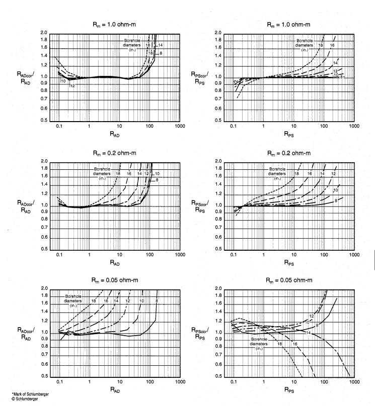
The CDR Compensated Dual Resistivity tool, a logging-whiledrilling (LWD) electromagnetic propagation tool, provides measurements with similarities to the medium (IM) and deep (ID) wireline induction logs. The phase shift and attenuation of
