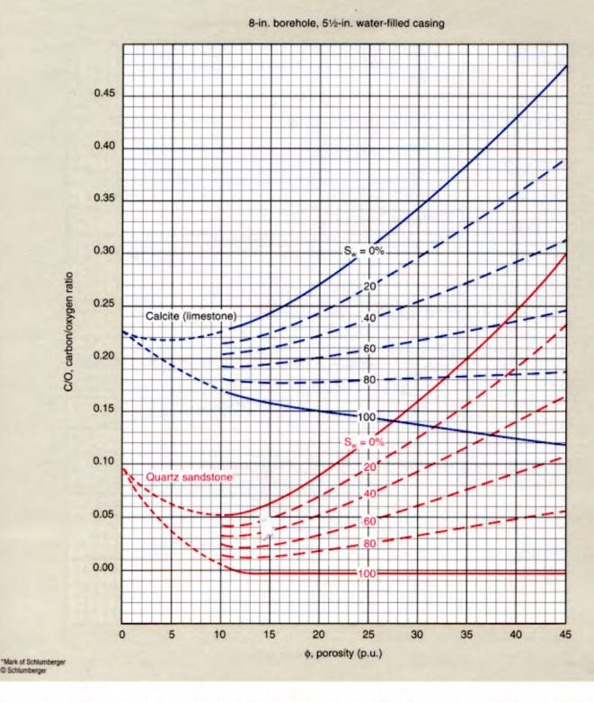
These charts permit the determination of water saturation from carbon/oxygen (C/O) ratio measurements made with the GST Induced Gamma Ray Spectrometry Tool in inelastic mode operation.
