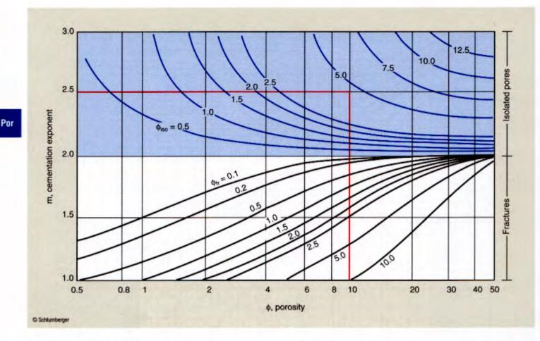
Chart Por-1a is based on a simplified model that assumes there is no contribution to formation conductivity from vugs and moldic porosity, and that the cementation exponent, m, of fractures is 1.0.
