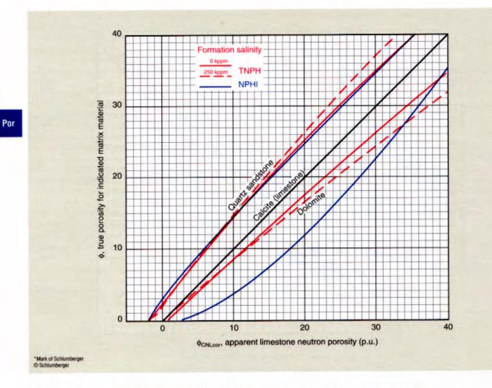
Chart Por-13b can be used in the same way as Chart Por-13a, on the previous page, to convert CNL porosity logs (TNPH or NPHI) from one lithology to another. If a log is recorded in limestone porosity units in a pure quartz sandstone formation, the true porosity can be derived.
