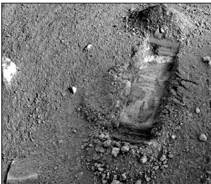
True colour photo image of a Mars Phoenix trench. White areas are believed to be water ice, as they appear to sublimate slowly after exposure to the Martian atmosphere. Samples were processed in the Thermal Evolved Gas Analyzer (TEGA).
