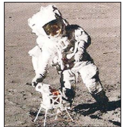
Harrison "Jack" Schmidt deploying the Surface Electrical Properties equipment (SEP) during Apollo 17 mission, 1972.
