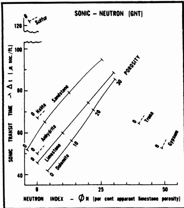
Fig. 18-2 — Sonic-Neutron crossplot for mineral identification. (Courtesy SPWLA, Ref. 9)
