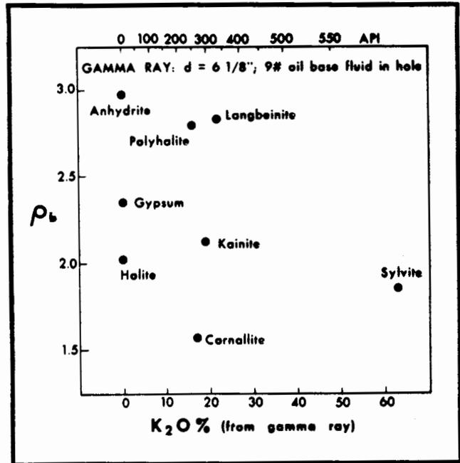
Fig. 18-3 — Crossplot of bulk density and apparent K<sub>2</sub>O content (from Fig. 18-4) identifies potash minerals. (Courtesy SPWLA, Ref. 9)
